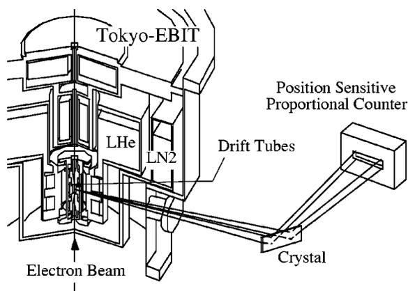
FIG. 1. Diagram of the experimental arrangement. Neonlike ions were produced and trapped at the center of the drift tubes. The spectrometer was operated *in vacuo*, although the vacuum chambers are not shown.
