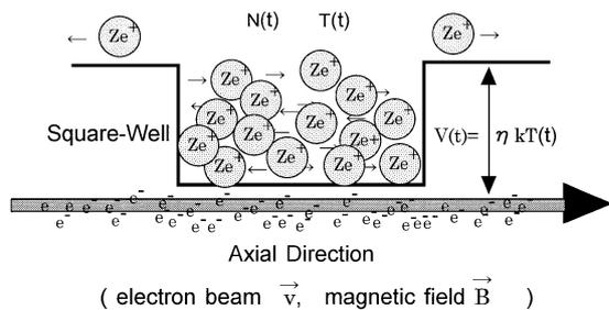
Fig. 1. Axial-escape and same charge-state model of pulsed evaporative cooling for highly charged ions in an EBIT.
